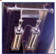
Two double-acting air cylinders activate the system in both directions.
