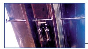
A 1 1/4 solid steel shaft moves both arms simultaneously, ensuring synchronized movement each time.
