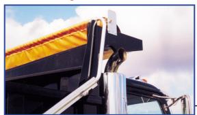
A 3 spring-loaded roller ensures a smooth operation. It keeps the tarp taut and in the covered postion as the tarp returns.
