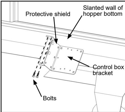
**Option 3 -** Mounting to slant of hopper bottom
