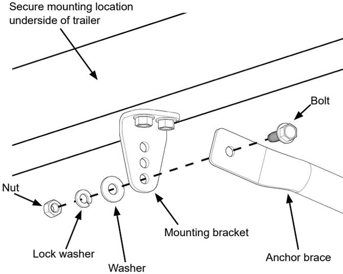
B. With anchor brace held in place make a mark at location shown. Remove brace and cut off excess at mark.
