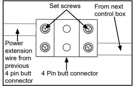
J. Connect extension wires to last 4 pin butt connectors (on control box wire side), then slide heat shrink over power extension wires.
